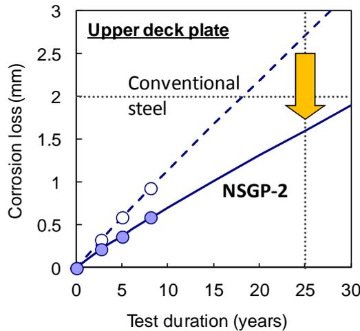
Fig. 11: Results of the exposure test on the upper deck of an Aframax tanker
