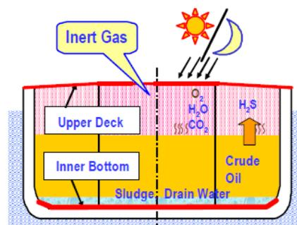
Fig. 1: Corrosion environment of COT
