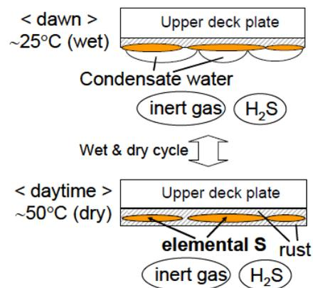
Fig7: Corrosion mechanism at the upper deck of COT
