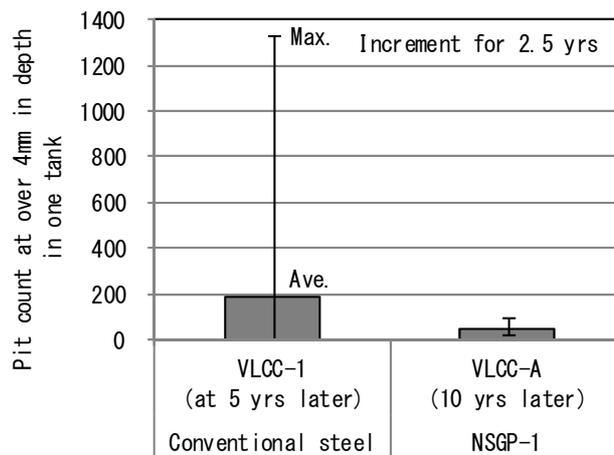
Fig. 3: Observed pit count at over 4 mm in depth for NSGP-1 VLCC and conventional VLCCs
