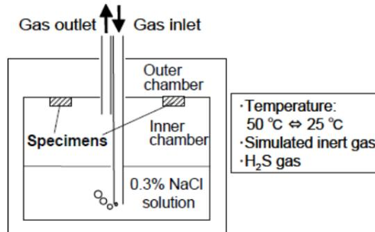
Fig. 8: Simulated corrosion test apparatus for the upper deck of a COT
