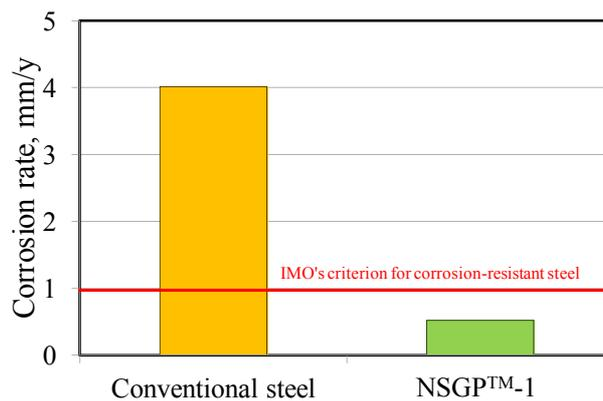
Fig. 2: Corrosion test results of the developed steel and conventional steel as per IMO Resolution MSC.289(87)
