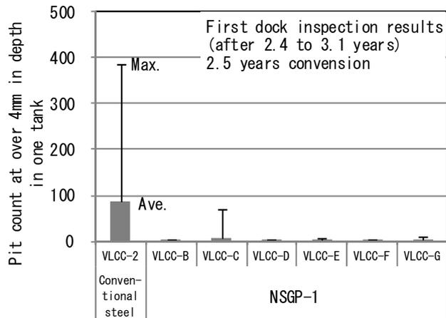
Fig.4: Observed pit count at over 4 mm in depth for the six VLCCs that used NSGP-1 and for conventional VLCC
