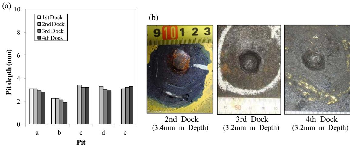
Fig.6:(a) Pit depth at the first, the second, the third and fourth dockings. (b) Appearances of pit “c” at the second, the third and fourth docking.
