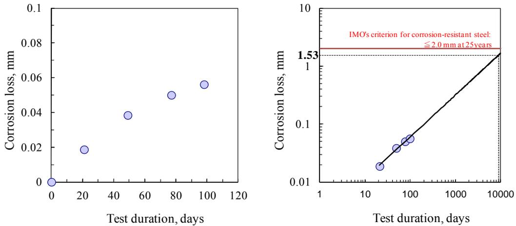
Fig. 10: Corrosion test results of NSGP-2
