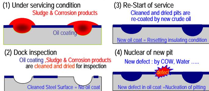
Fig.5: Mechanism of pit termination at dock inspection [2].
