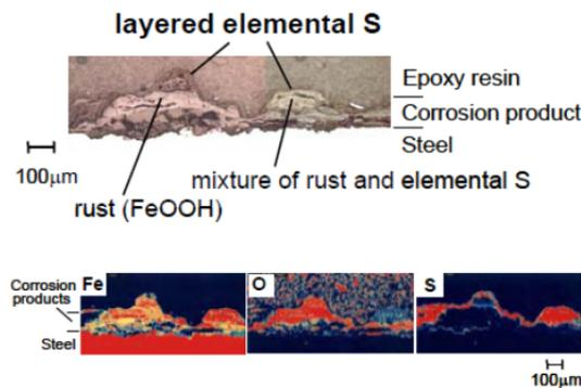
Fig. 9: Cross sectional morphology and distribution of elements by the Electron Probe Microanalysis in the corrosion products of specimen after a simulated corrosion test for the upper deck
