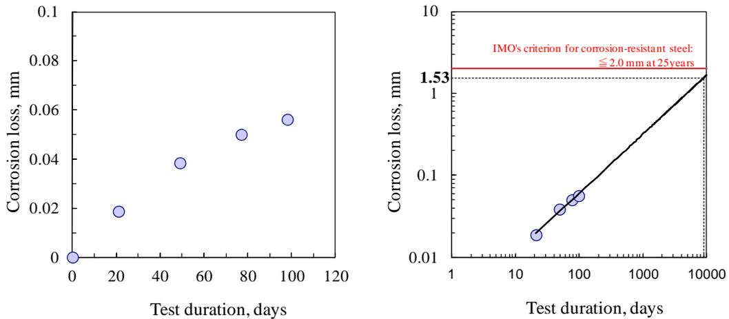
Fig. 9: Corrosion test results of NSGP™-2
