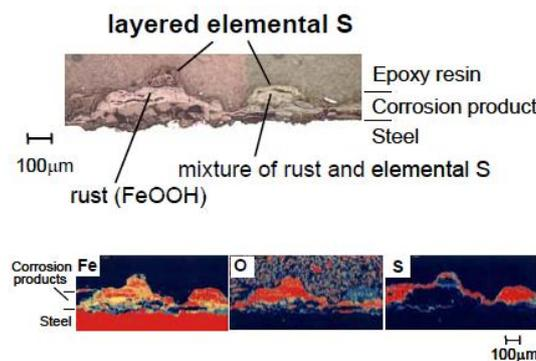
Fig. 8 Cross sectional morphology and distribution of elements by the Electron Probe Microanalysis in the corrosion products of specimen after a simulated corrosion test for the upper deck
