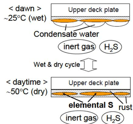
Fig.6: Corrosion mechanism at the upper deck of COT
