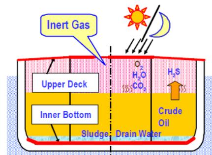
Fig. 1: Corrosion environment of COT
