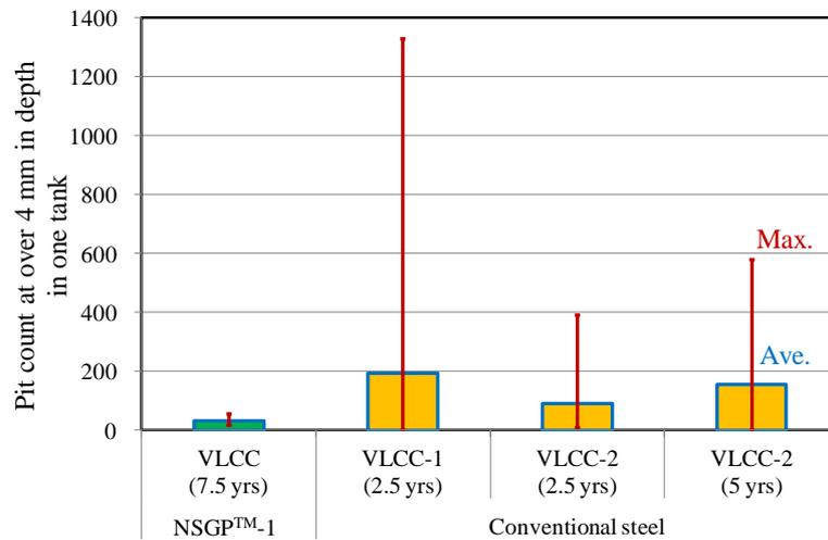
Fig. 3: Observed pit count at over 4 mm in depth for CRS VLCC and conventional VLCCs
