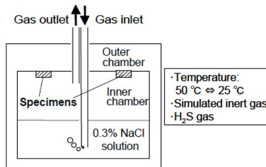
Fig. 7 Simulated corrosion test apparatus for the upper deck of a COT
