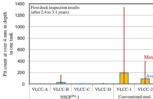
Fig.5: Observed pit count at over 4 mm in depth for the four VLCCs that used NSGP™-1 and for conventional VLCCs
