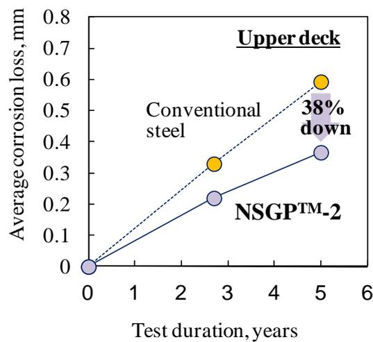
Fig. 10: Results of the exposure test on the upper deck of an Aframax tanker
