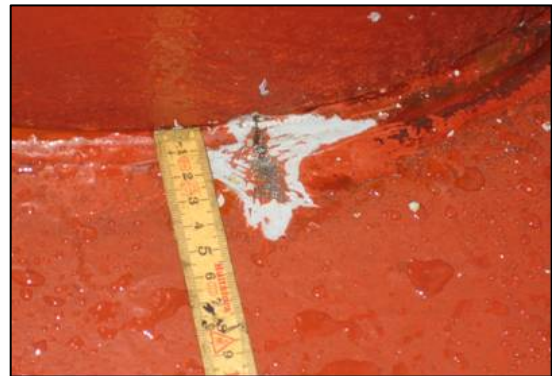
Close-up showing crack in deck plating
