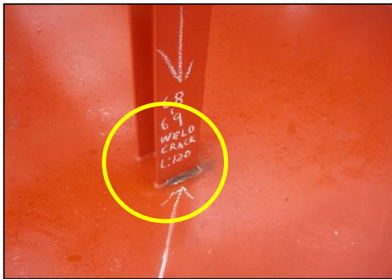
Crack i.w.o fillet welding i.w.o pipe support connection to upper deck.
