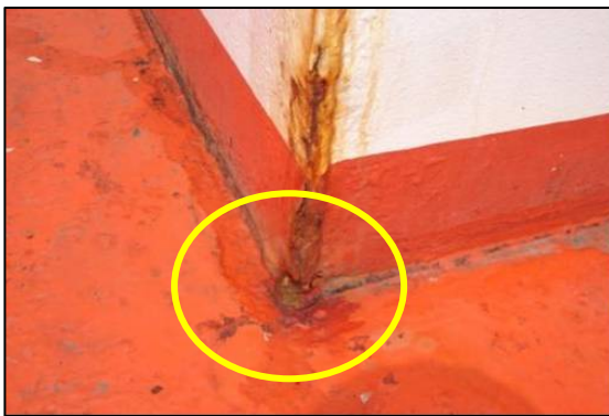
Deckhouse corner at connection to upper deck. Note crack in way of fillet welding and local scale
