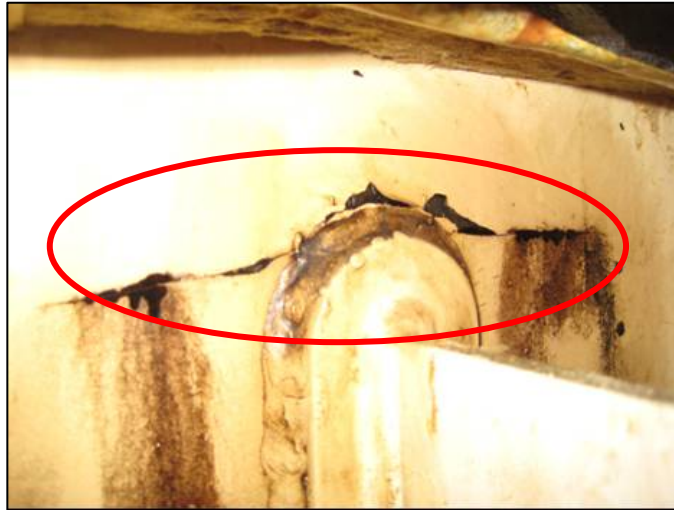
Crack in way of ladder lug doubler – connected to unsupported plate of oil tank. Vibration induced crack
