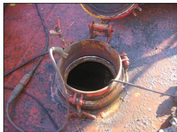
Butterworth hatch modified to ensure welding is clear of deck opening.
