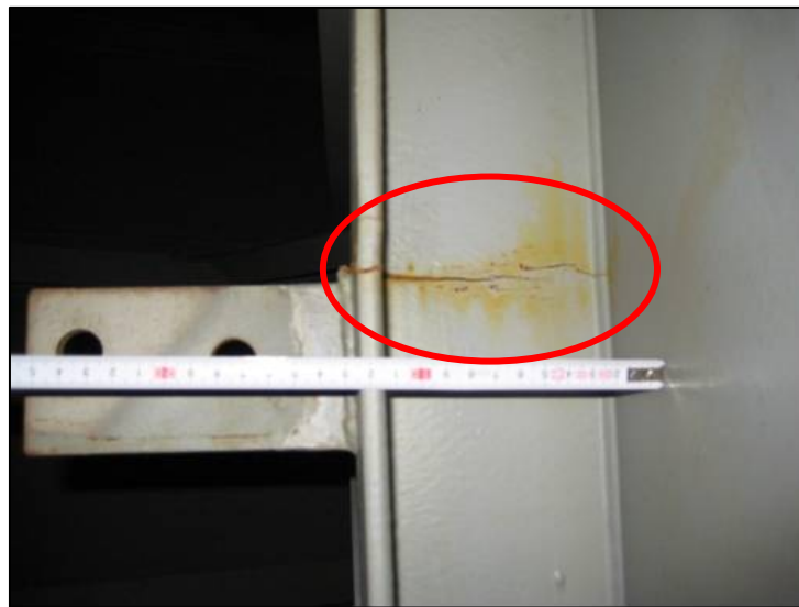
Non structural staging lug in fresh water tank. Abrupt connection and poor return weld detail resulted in the crack shown – vibration induced crack
