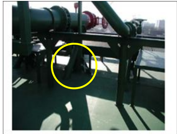
Cracks at the pipe support bracket connection to main deck toe
