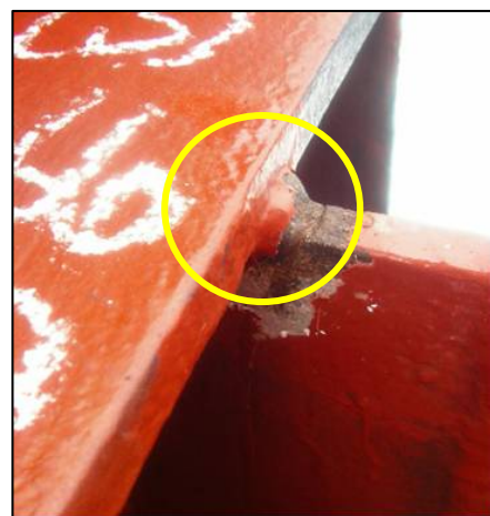
Gutter bar cracked in way of connection to mooring fairlead.
