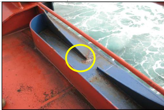
Paint disturbance noted in way of gutter bar taper toe
