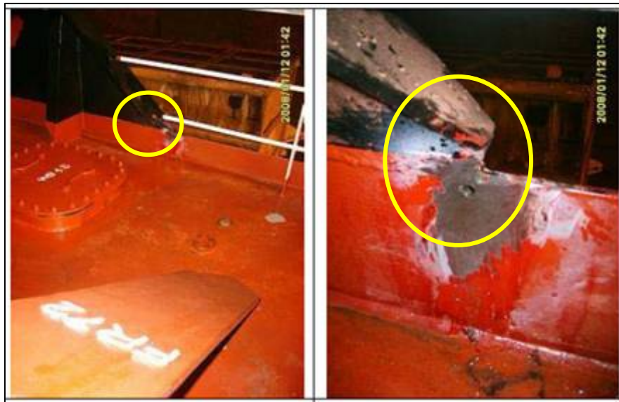
Crack developed through the sheerstrake at the manifold resting support.
