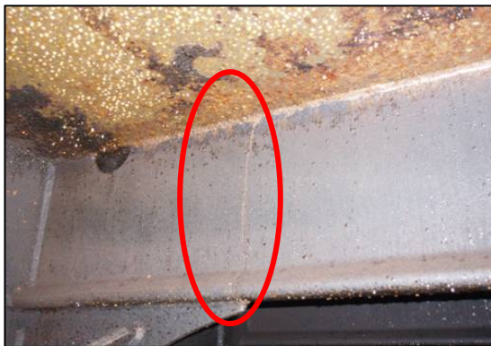
Crack in way of local underdeck girder end bracket toe
