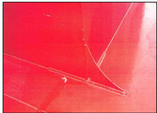
Deckhouse corner welding repaired and soft bracket fitted
