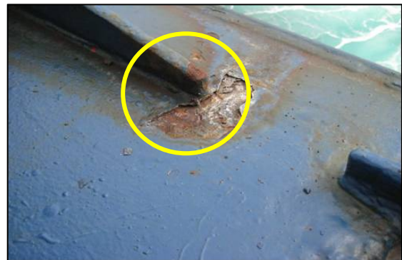
Upper deck plate crack in way of gutter bar taper toe
