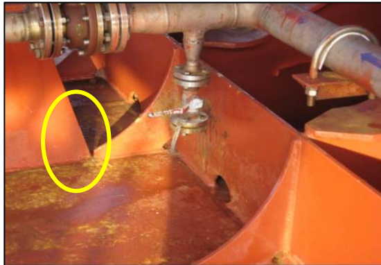
Deck machinery coaming bracket erroneously trimmed hence creating excessive toe height. Crack in deck plate resulted
