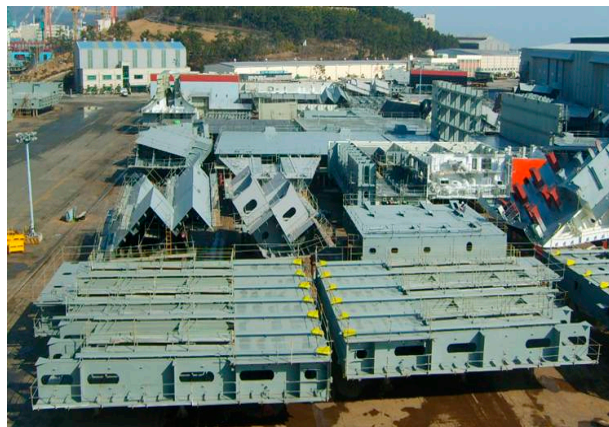
Fig.2 Block stock area for final touch-up and inspection
