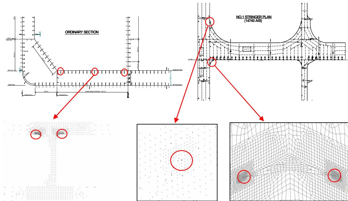
Fig. 7 Locations of low cycle fatigue analysis
