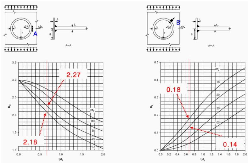
(a)  $K_g$  at hole with inserted tubular.
