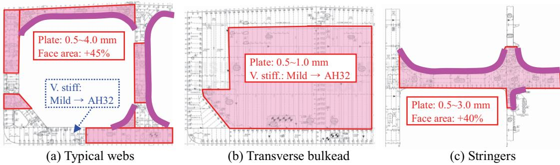
Fig. 9 Reinforcement for transverse member
