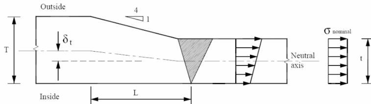
**Fig. 5 SCF for butt connection with misalignment**
