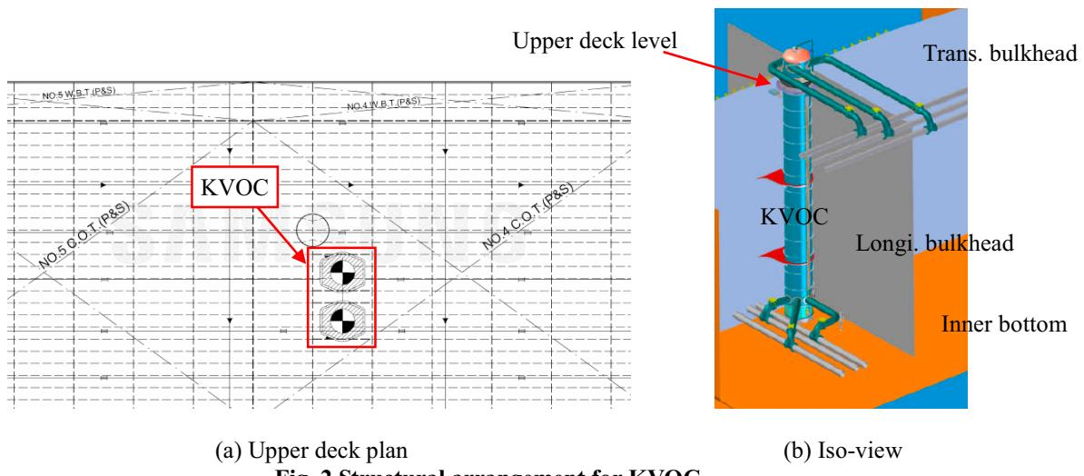
**Fig. 2 Structural arrangement for KVOC**
