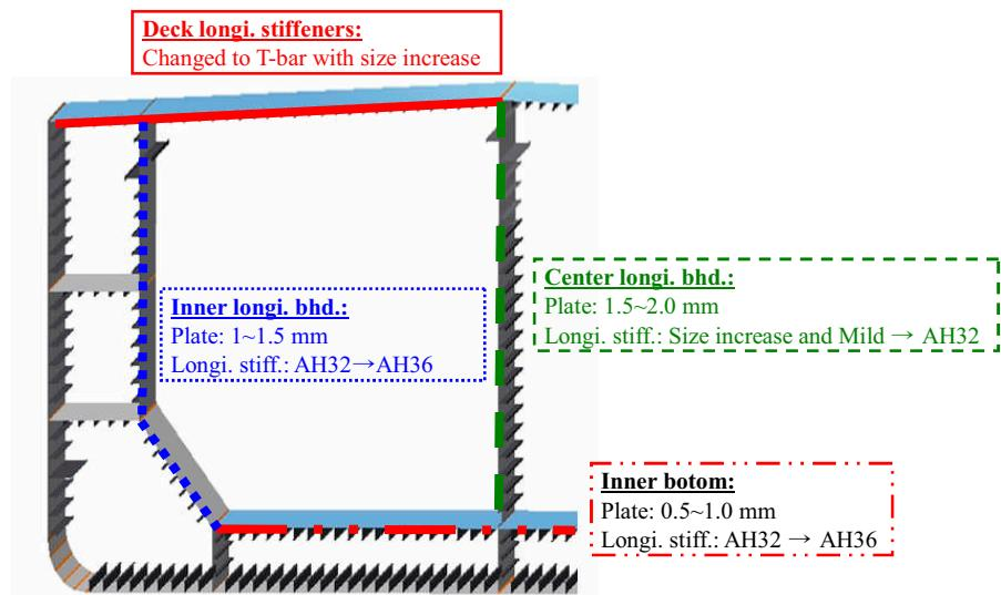
Fig. 8 Reinforcement for longitudinal members
