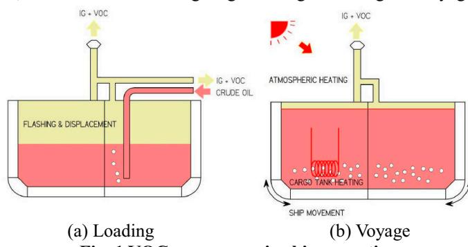
**Fig. 1 VOC occurrence in ship operation**
