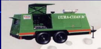
NLB Corp. Ultra Clean 36K (USA) Max. capacity of 2500 bar
