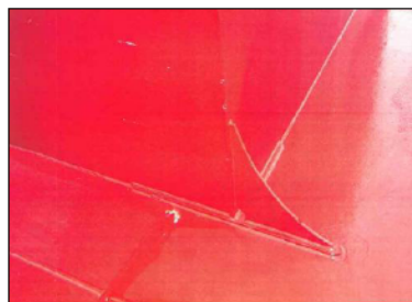
Deckhouse corner welding repaired and soft bracket fitted.
