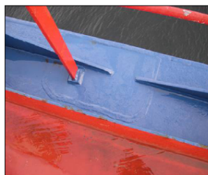
Upper deck repair / gutter bar taper toe "nose" minimum height
