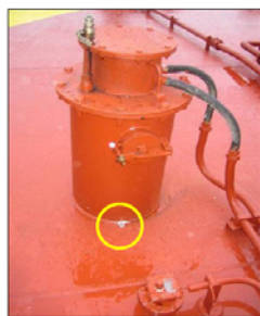
Radar contents gauge pedestal. Note paint disturbance at pedestal connection to the upper deck.
