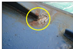
Upper deck plate crack in way of gutter bar taper toe
